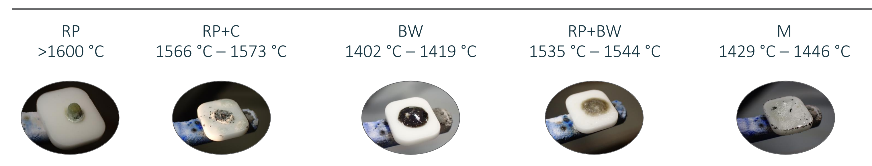
Melting interval expressed as the flow temperature with specimen appearance after thermal treatment in the HM
