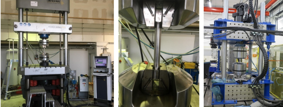
Fig. 3: Resonance test rig, clamped sample, servo-hydraulic test rig
