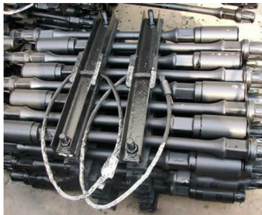
Figure 14: Steel frame with plastic separators and bolts screwed together at the top 112
