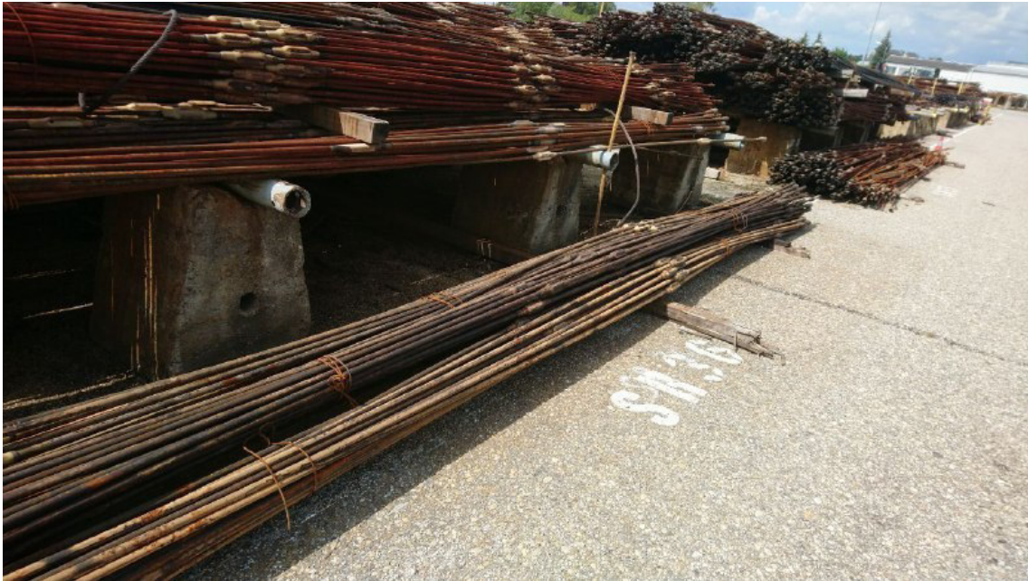
Figure 29: Buffer storage area for all sucker rods of batch D-25%
