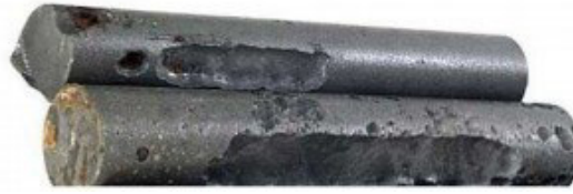
Figure 11: CO 2 corrosion on sucker rods 87
