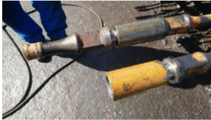
Figure 25: Caliper and sleeve for checking threads
