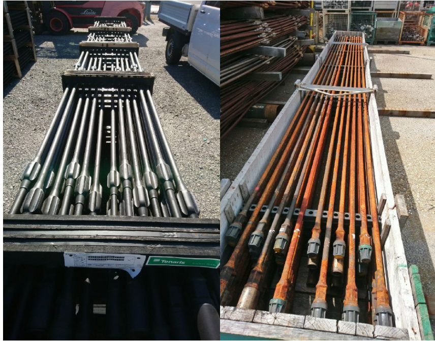
Figure 15: Transport and storage solutions for sucker rods at OMV pipe yard in Prottes
