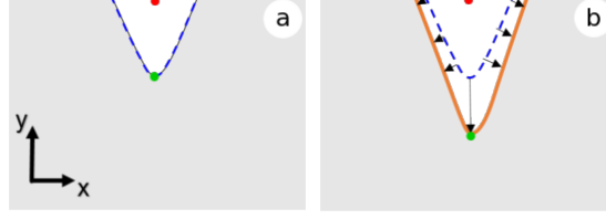
Figure 28: Schematic crack flank detection on consecutive frames: a) Previous frame with the located crack flank (dashed blue line). b) Following frame with the previously found crack flank (dashed blue line), a possible found contour line (orange solid line), representative distance measure between previous crack flank and contour line for all pixels on that contour line (black arrows), reference point for measurement (red dot) and the possible crack tip (green dot).
