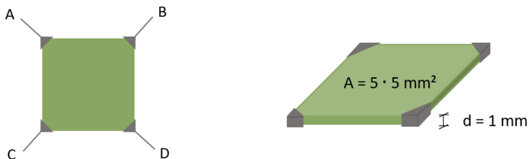
Fig 3.7 Arrangement of the contacts in four-point van der Pauw geometry.
