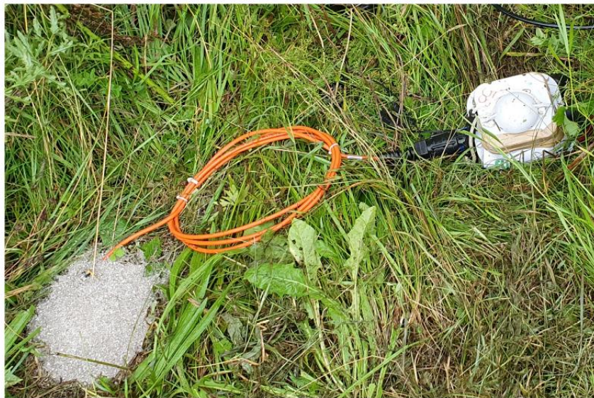
Figure 11: DSU3-SA covered with sand and RAU-D deployed in a field outside the mine.
