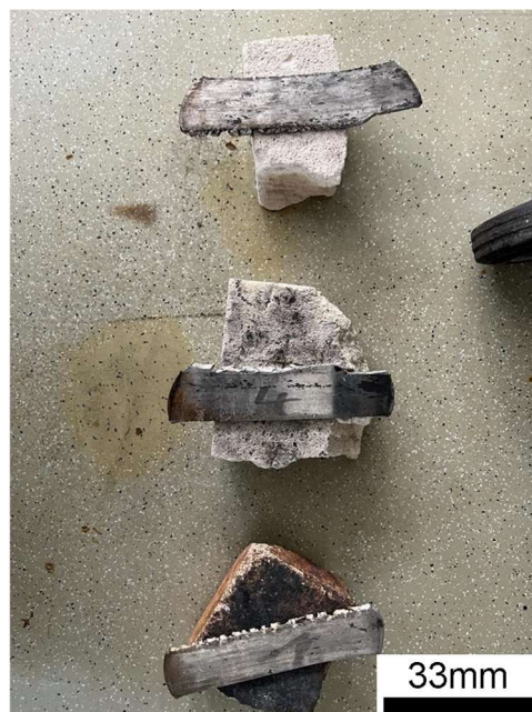
Figure 3-12: The 5 mm specimens after 340 °C rolling
