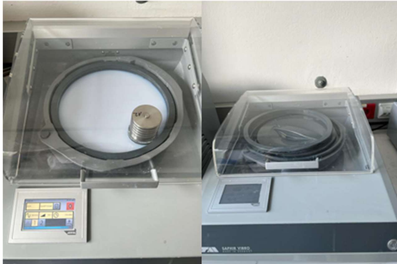
Figure 3-18: Vibration polishing (ATM Saphir Vibro).
