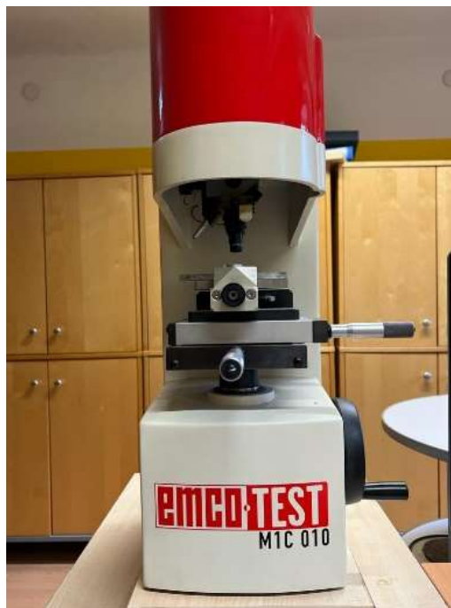
Figure 3-14: The Vickers machine at the Chair of Metal Forming.
