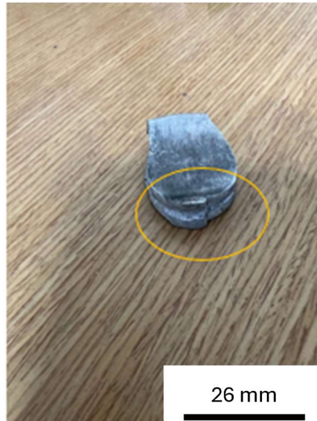
Figure 3-9: Crack after cold rolling.
