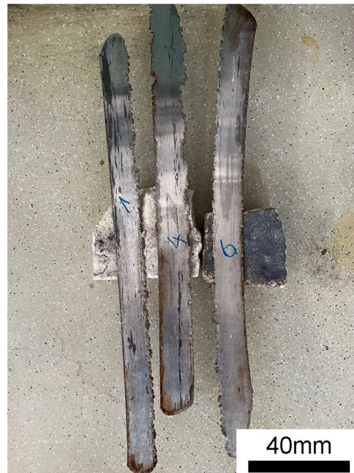
Figure 3-13: The 1 mm specimens after 340 °C rolling
