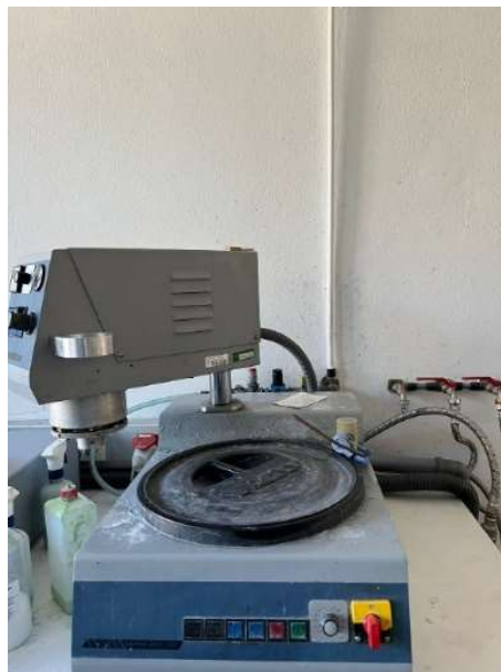
Figure 3-15: Grinding machine ATM Saphir 350.
