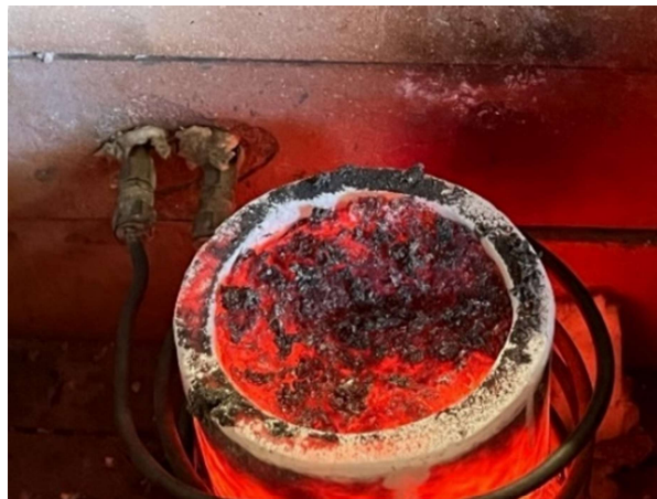
Figure 3-3: Unsolved SiC in the induction melting.
