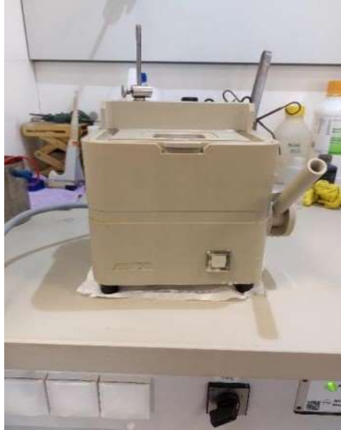
Figure 3-16: Barker etching (ATM Kristall 620).
