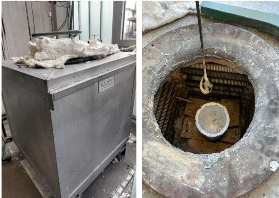
Figure 3-4: Nabertherm crucible furnace at the Chair of Casting Research.
