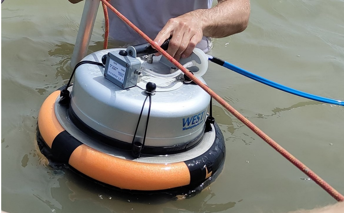
Figure 16: Bell-shaped device that stored the gas which enabled sampling and measurement of the collected gas.
