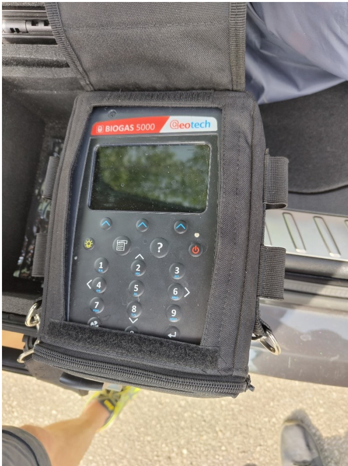
Figure 14: Gas analyse device on site that was used to analyse, collect and transfer the gas into the gas sampling bags.
