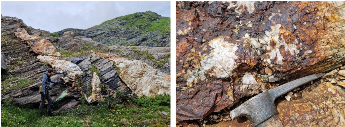
Figure 12: Left: Pasterze to the west of the Margaritzen reservoir with a view to the west. Two large (up to > 1 m) quartz veins with sulfide mineralization. Right: Close-up of the left quartz vein with visible pyrite mineralization and reddish-brown weathering material covering the quartz.
