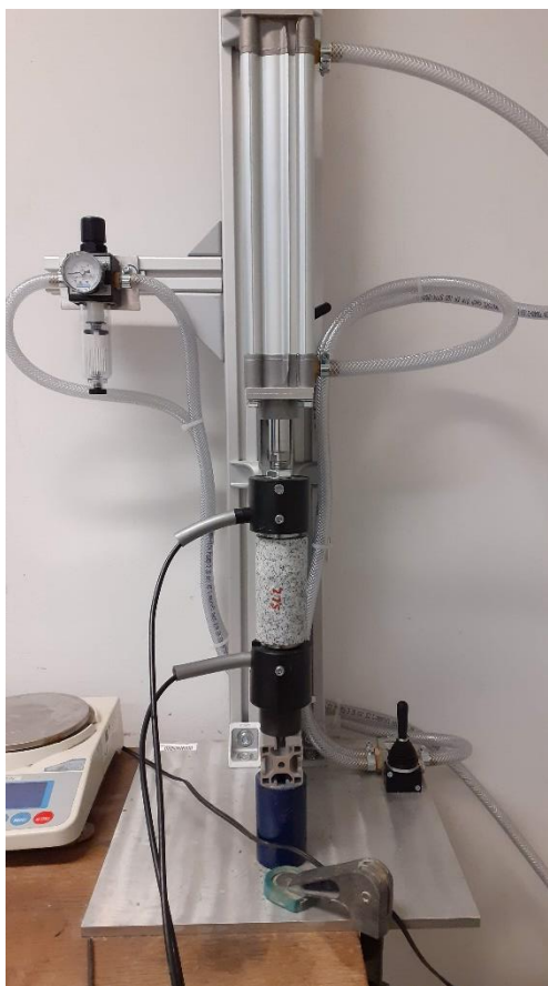
Figure 15: Geotron Elektronik ultrasonic generator USG 40 used for the measurements (R. Winstel)
