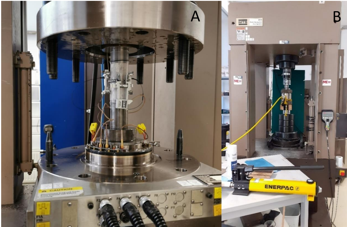
Figure 12: Setup of the TCS testing with a triaxial testing setup of MTS (R. Winstel) (A) and Hoek Cell, photo taken by Marlene Villeneuve (B)
