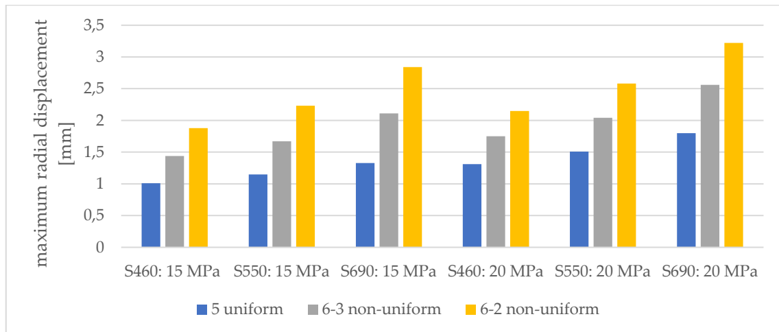
Figure 84: Maximum radial displacement of the steel lined storage boundary with steel grades S460, S550 and S690 for Sauburger Kalk, different uniform and non-uniform in-situ stress conditions as well as a p_i of 15 and 20 MPa
