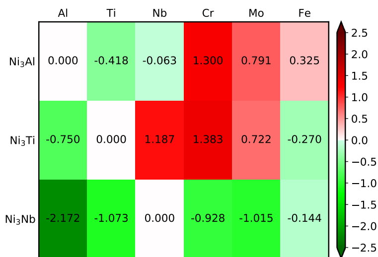
Fig. 9.3 The solution energy (in eV) heat map for L1_2 - Ni_3X ( X=Al, Ti, Nb ) intermetallic compounds. Green blocks represent solutes with negative solution energies and red blocks represent solutes with positive solution energies on the preferred sublattice chosen according to the results on the transfer energies shown in Figure 9.2.
