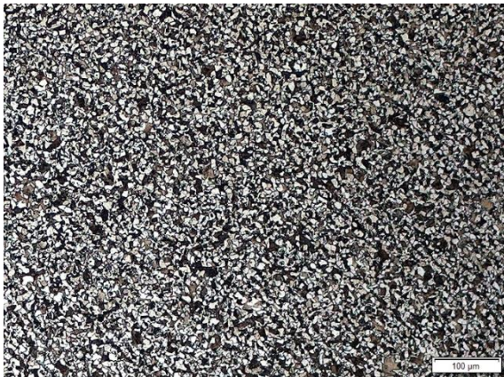
Figure 11: 27MnSiVS6 (as-rolled), transverse section 100x magnification
