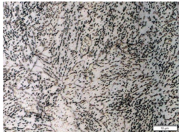
Figure 16: 42CrMo4 (annealed), transverse section 1000x magnification
