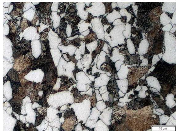
Figure 14: 27MnSiVS6 (as-rolled), transverse section 1000x magnification
