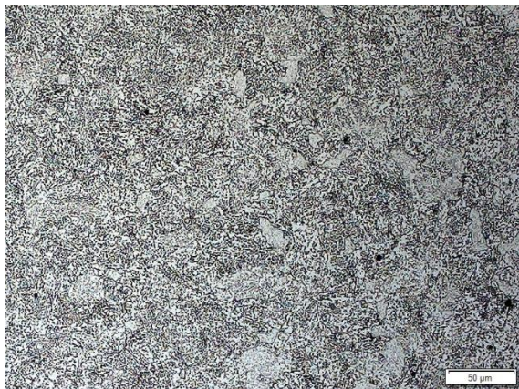
Figure 15: 42CrMo4 (annealed), transverse section 200x magnification
