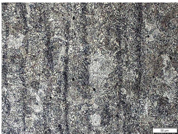
Figure 17: 42CrMo4 (annealed), longitudinal section 200x magnification
