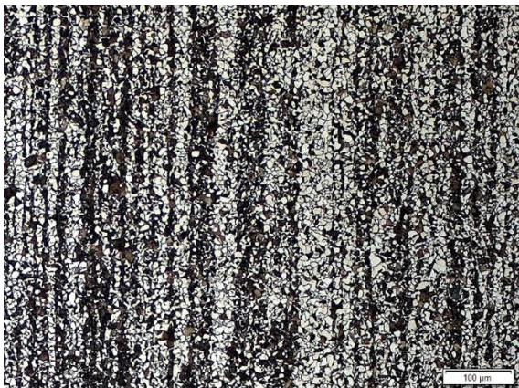
Figure 13: 27MnSiVS6 (as-rolled), longitudinal section 100x magnification
