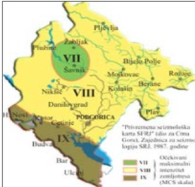
Figure 18. Seismic regionalization of the territory of Montenegro. Source: Seismological Observatory of Montenegro
