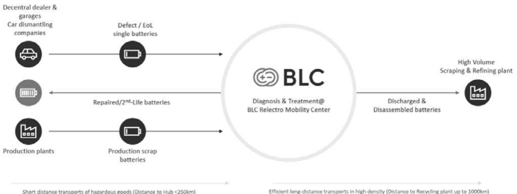
Fig. 3: holistic overview of hub concepts that improve efficiency and enable scalability for low-volume processes
