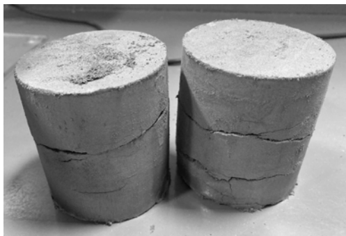
Fig. 2: Briquettes produced with grinding sludge (Source: own picture)
