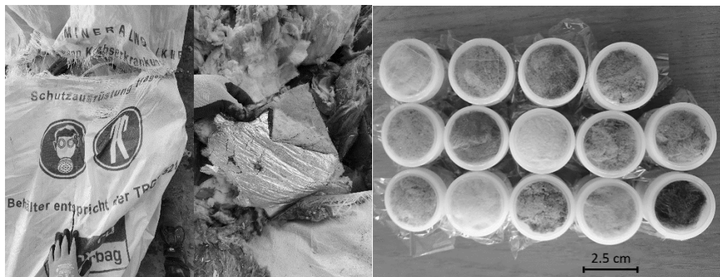
Fig. 1: Mixed mineral wool waste (L); separated mineral wool waste samples (R)
