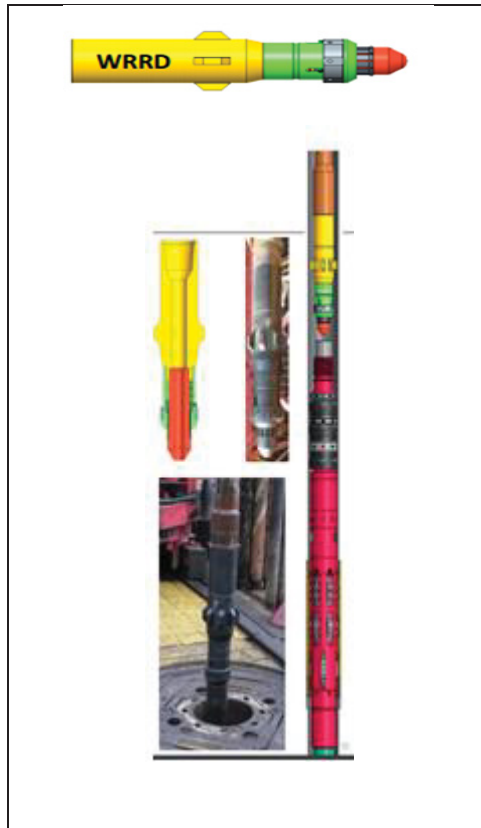
Figure 11: Working Release Retrieval Device (WRRD) (17)
