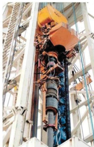
Figure 8: Casing Drive System (14)
