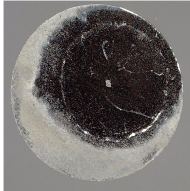
Figure 14: HPT sample used both for electron-microscopy investigations and in situ TEM heating experiments.
