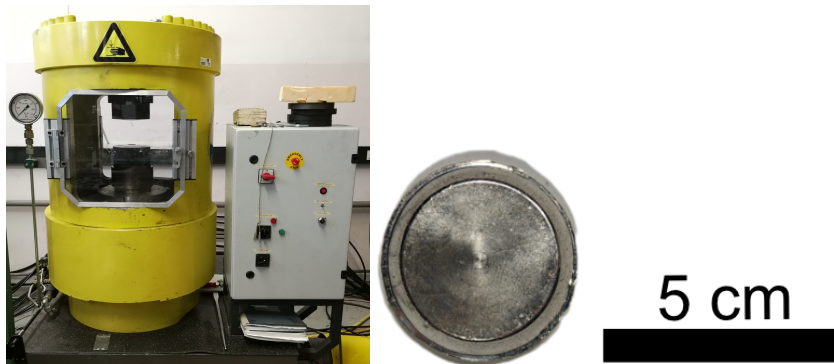
Figure 12: HPT equipment for synthesis of UFG AA6061 alloy and the final shape obtained after the HPT processing.
