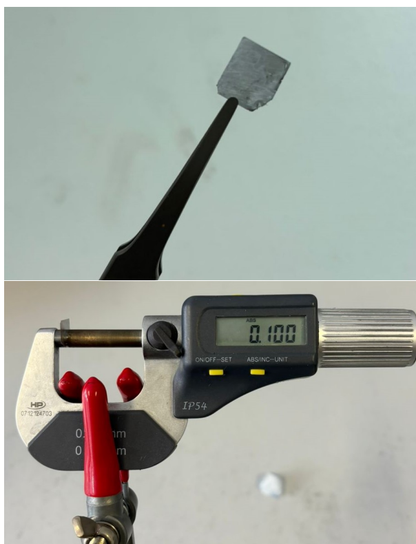
Figure 13: Foils prepared with 100\ \mu\text{m} after mechanical polishing.
