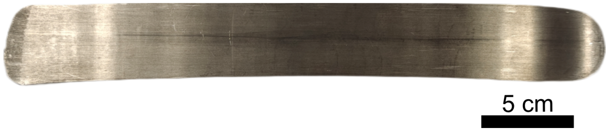
Figure 11: Final shape of the CG AA6061 alloy after homogenisation, hot- and cold-rolling prior HPT.
