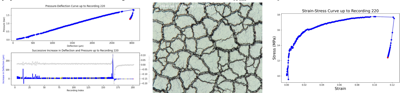
(e) Crack pattern stays constant \epsilon_{total} = \epsilon + \epsilon_0 = 11.484\% + 1.051\% = 12.535\%
