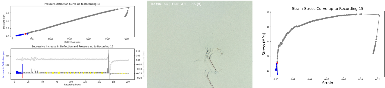
(b) First crack initiation at at \epsilon_{total} = \epsilon + \epsilon_0 = 0.15\% + 1.051\% = 1.201\%
