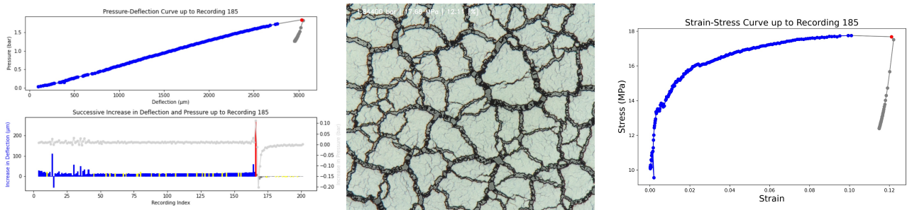
(d) Point of material failure (rip) with visible stress relief \epsilon_{total} = \epsilon + \epsilon_0 = 12.215\% + 1.051\% = 13.266\%
