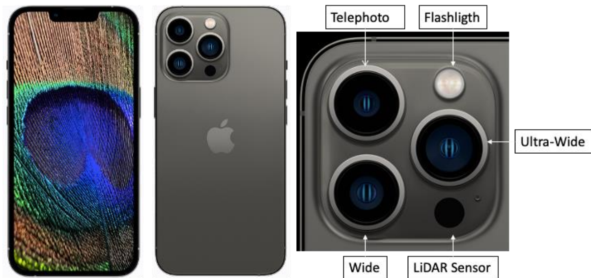
Figure 4: iPhone 13 Pro and its camera system in detail 34 . The device presents a camera system with three different cameras allowing for an advanced image stabilization and several aperture ranges. Furthermore, the smartphone is equipped with a regular flashlight and a LiDAR Sensor, enabling the performance of laser scanning.
