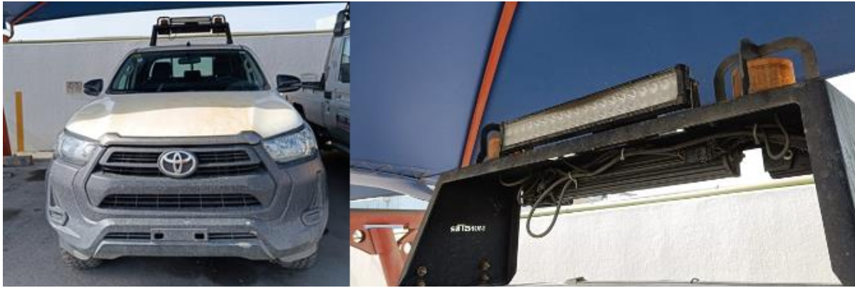
Figure 10: Toyota Hilux light system used to provide lighting in the performance of the laser scans.
