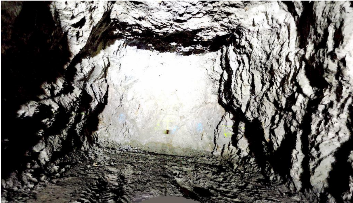
Figure 33: Visualization of Model 2 in Unity Scene. This model consists of the mesh generated from the point cloud captured with the TLS method.
