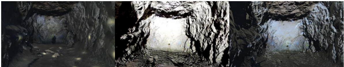
Figure 35: screenshot of the different VR models created using MLS with iPhone 13 Pro and TLS with Faro Focus S70. Panel A) consists of model 1, created from the iPhone 13 Pro scan; Panel B) is model 2, created from the Faro Focus S70 scan, without diminishing the point density; Panel C) is model 3, obtained by constructing a low-poly mesh in Blender, from the scan conducted with the Faro Focus S70.
