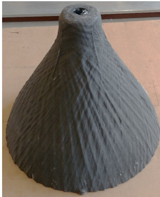
Figure 32: Result of VAP-infusion of dry-wound nosecone
