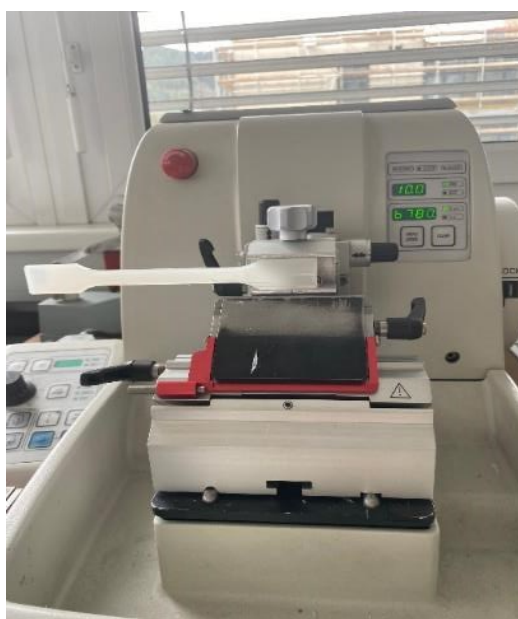
Fig. 3.3: PP-H clamped in the Leica RM 2255 microtome ready for slicing
