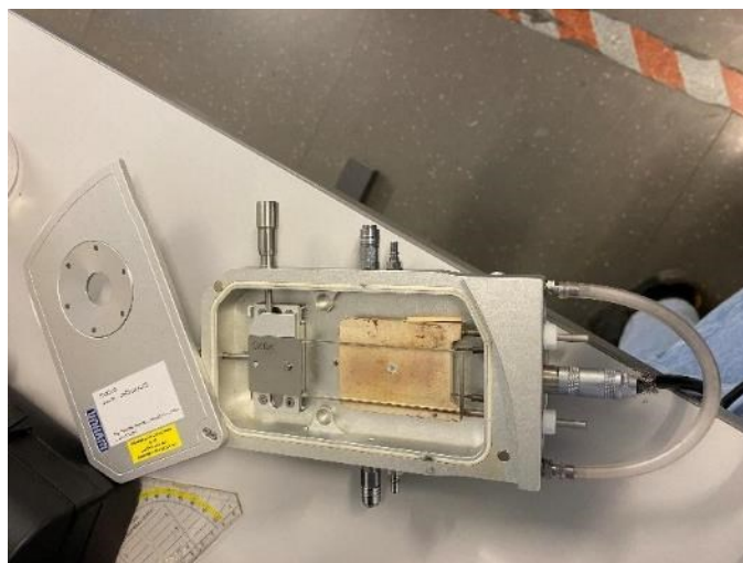
Fig. 3.4: Linkam 2028 Heating Stage for heating the PP samples
