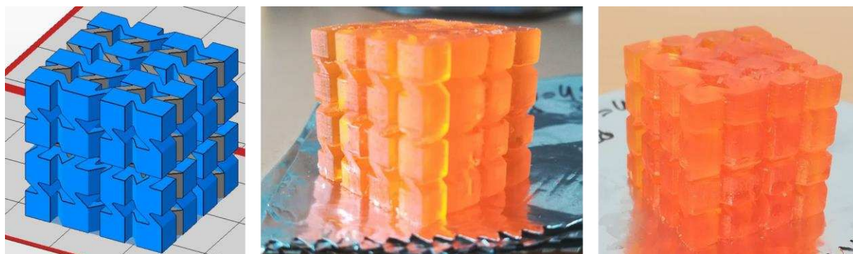
Figure S5. Multi-material test specimen fabricated via dual-wavelength DLP printing with dual resin-1-2. On the left side, the CAD data is shown with the color denoting the different wavelengths (blue: 365 nm, grey: 405 nm), in the middle and the right side the printed part is shown (sample dimensions: 20 mm x 20 mm x 20 mm).
