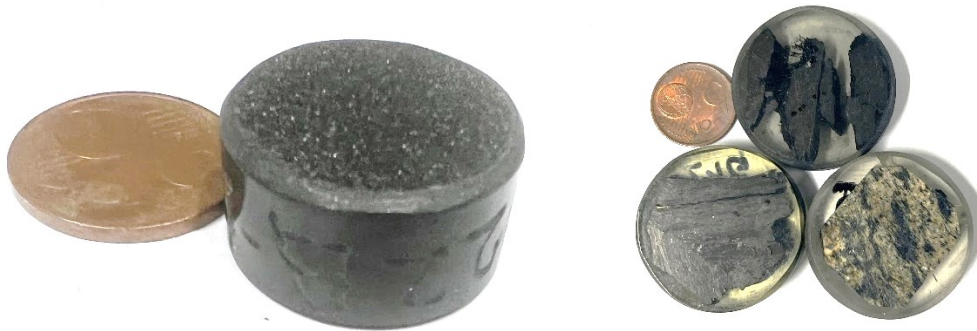
Figure 16: Graphite concentrates (left image) and raw ore (right image) embedded into epoxy resin
