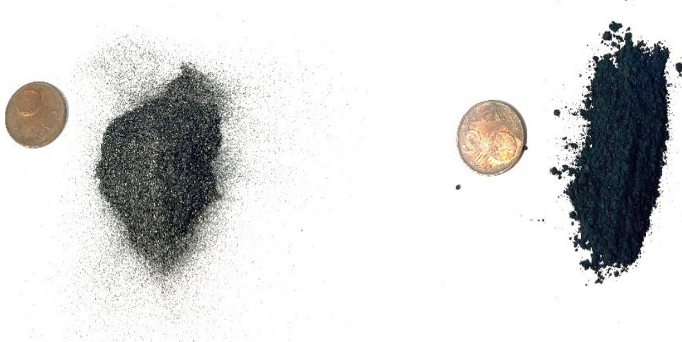
Figure 10: Flake (left) and amorphous (right) graphite concentrate
