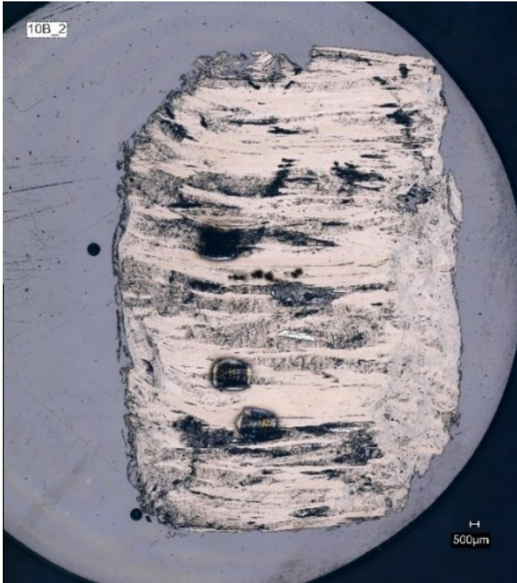
Figure 31: Highly pure vein graphite (lump ore) (yellowish-grey) sample 10B
