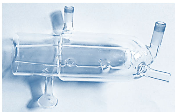
Figure 2-3 Scott spray chamber (Agilent Technologies, USA; source: E. Fasch).
