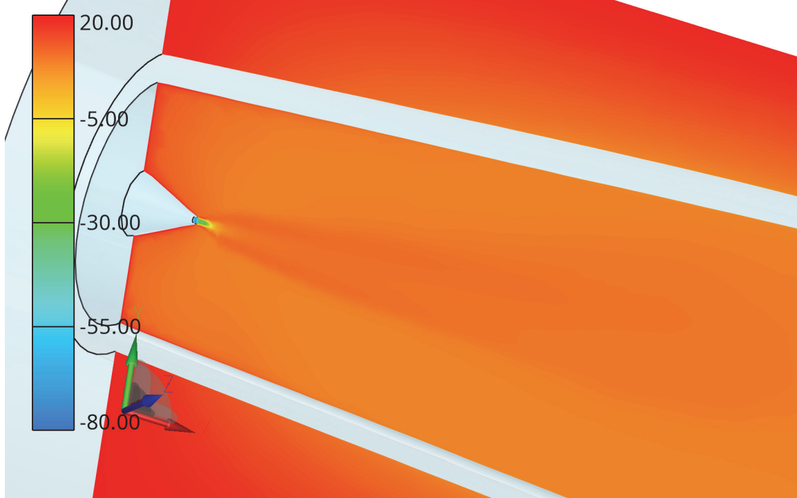
Figure 6-35 Temperature distribution in the Scott spray chamber at 20 °C (A) and in the inlet regime (B).
