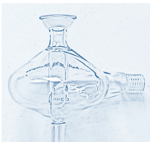
Figure 2-4 Cyclonic spray chamber (Agilent Technologies, USA; source: E. Fasch).
