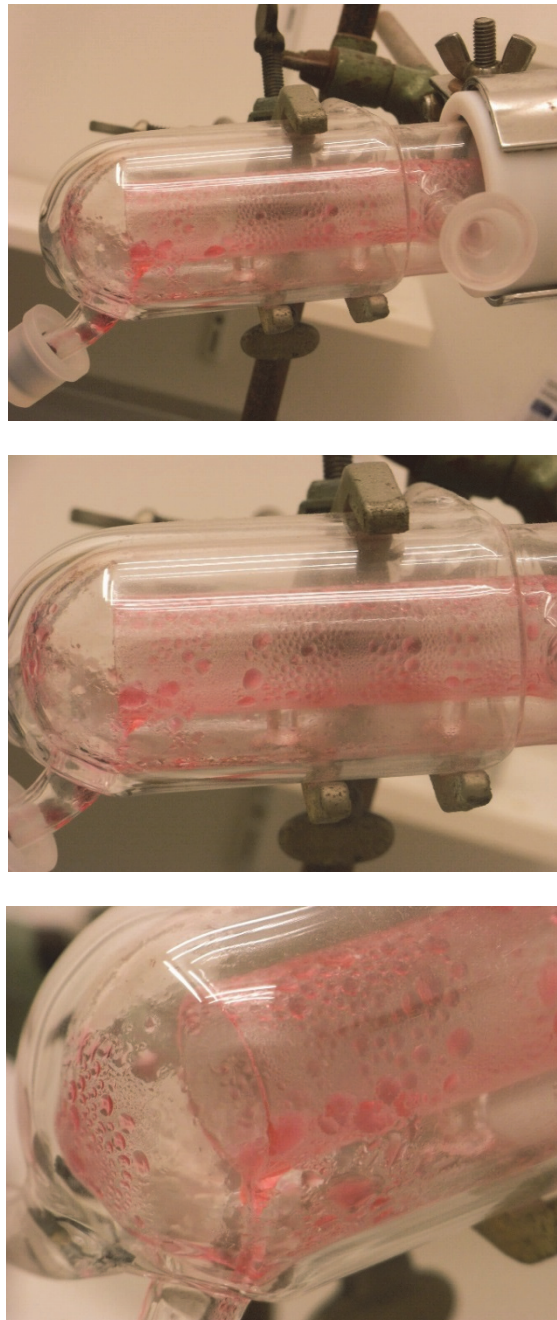
Figure 6-41 Pictures of the investigated double-pass glass spray chamber to evidence the zones of droplet impact, nebulizing a methylene red solution (source: E. Fasch).
