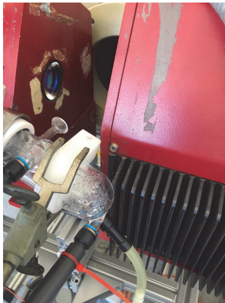
Figure 5-5 Top: Measurement principle of a Fraunhofer laser diffraction system by courtesy of Sympatec (© Sympatec GmbH); bottom: optical arrangement in the experiment (source: E. Fasch).
