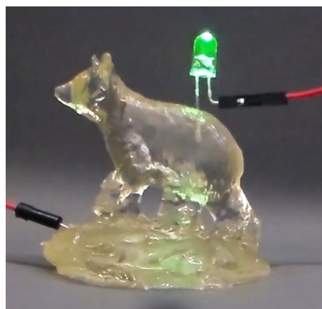
Figure 1.25 – A hydrogel-based bear structure was printed an electronic connector to demonstrate electric conductivity. 250 Copyright 2017 WILEY-VCH Verlag GmbH & Co. KGaA, Weinheim
