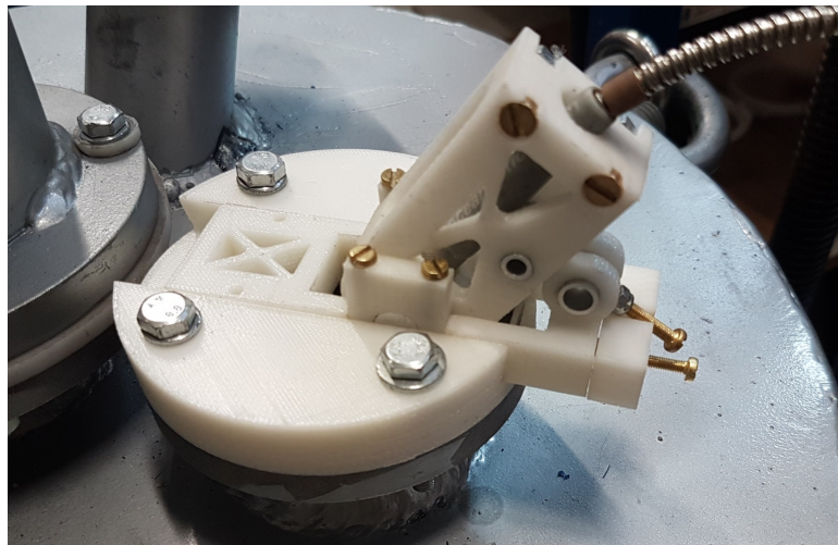
Figure 4.3: Fibre Holder Mounted on a Flange on Top of the Furnace Roof
