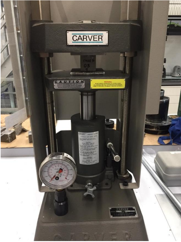
Figure 39 . Load Frame used to perform the UCS tests
