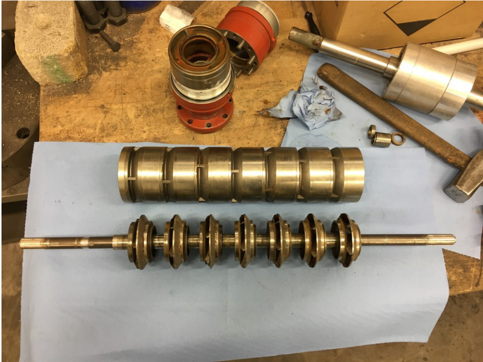
Figure 73: Dismantled REDA D2400N pump
