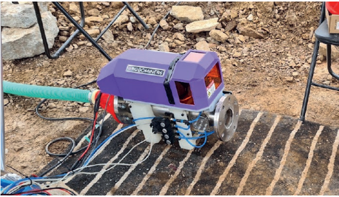
Fig. 12. Slurry spectrometer installed along the slurry transport line in the Kunda open pit mine (13).
