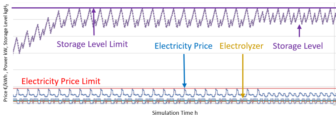
Figure 22: Exemplary evaluation of the hydrogen storage KPI, the electricity prices are below the electricity price limit, but the storage capacity limit is reached at several points.
