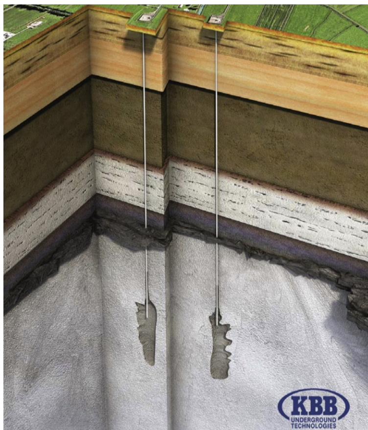
Figure 12: Artificial underground salt cavern [44].
