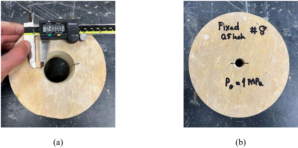
Figure 4.4: a) Limestone sample with 50.8 mm inner hole diameter b) Limestone sample with 12.7 mm inner hole diameter
