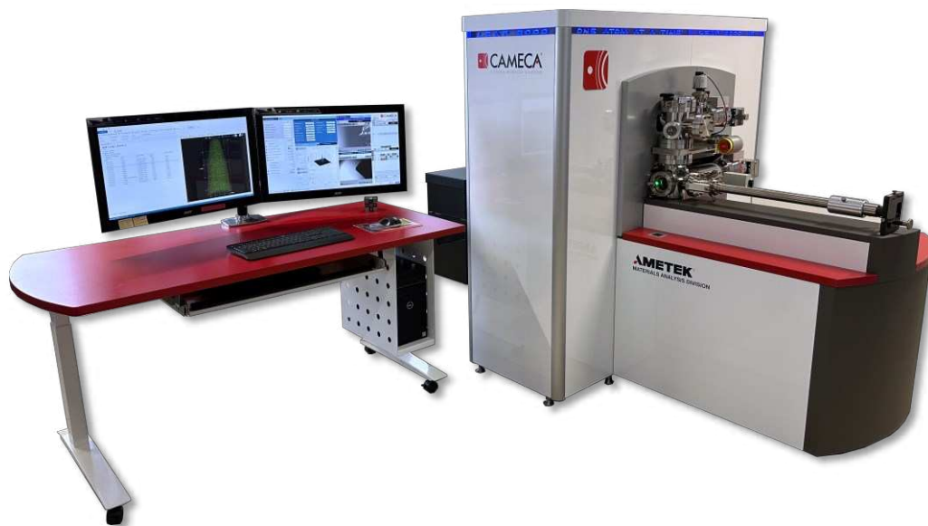
Fig. 1: Atom probe LEAP 5000 XR manufactured by CAMECA Instruments at the Department Materials Science.
