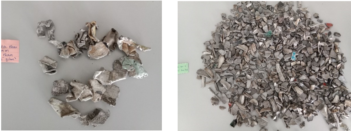
Figure 26 left image shows particles with the density class -2.5 \text{ g/cm}^3 to +1.4 \text{ g/cm}^3 and the right image shows the particle with the density class +2.5 \text{ g/cm}^3 to -3.0 \text{ g/cm}^3
