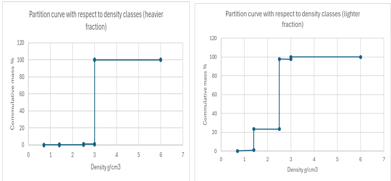
Figure 23 Graphs represent the recovery of materials in different density classes in -90mm +30mm sample.
