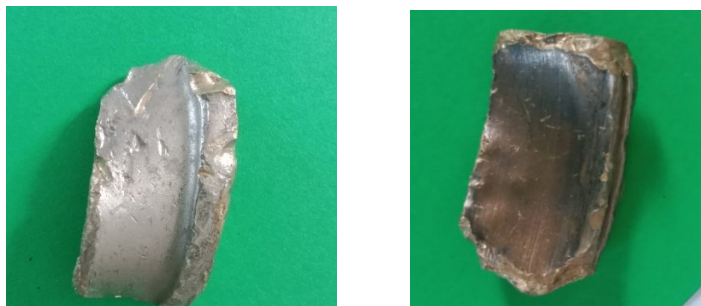
Figure 29 Images of the same particle with the coated and uncoated side showing huge variability in XRF results.
