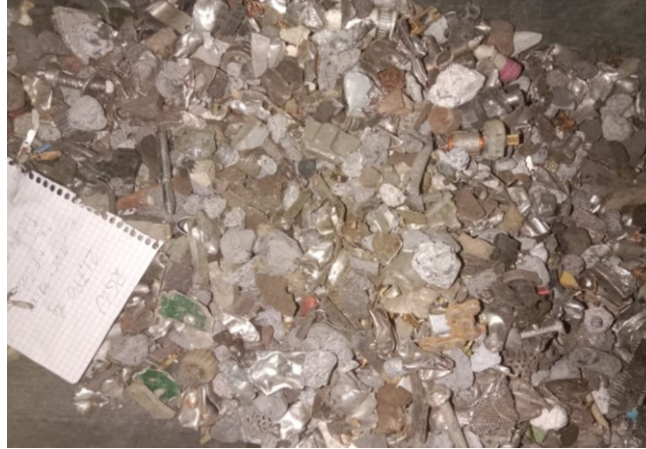
Figure 18 Image of the eddy current magnetic reject sample
