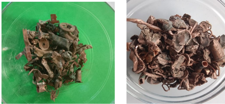
Figure 27 Left image shows particle of copper identified by XRF and right image shows particle of hand-sorted copper.
