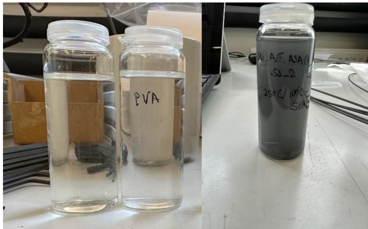
Fig. 48 Water debindable test of PVA (left) and PVA/ASA feedstock
