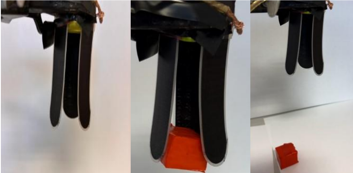
Figure 47: Working principle of the three-finger actuator.
