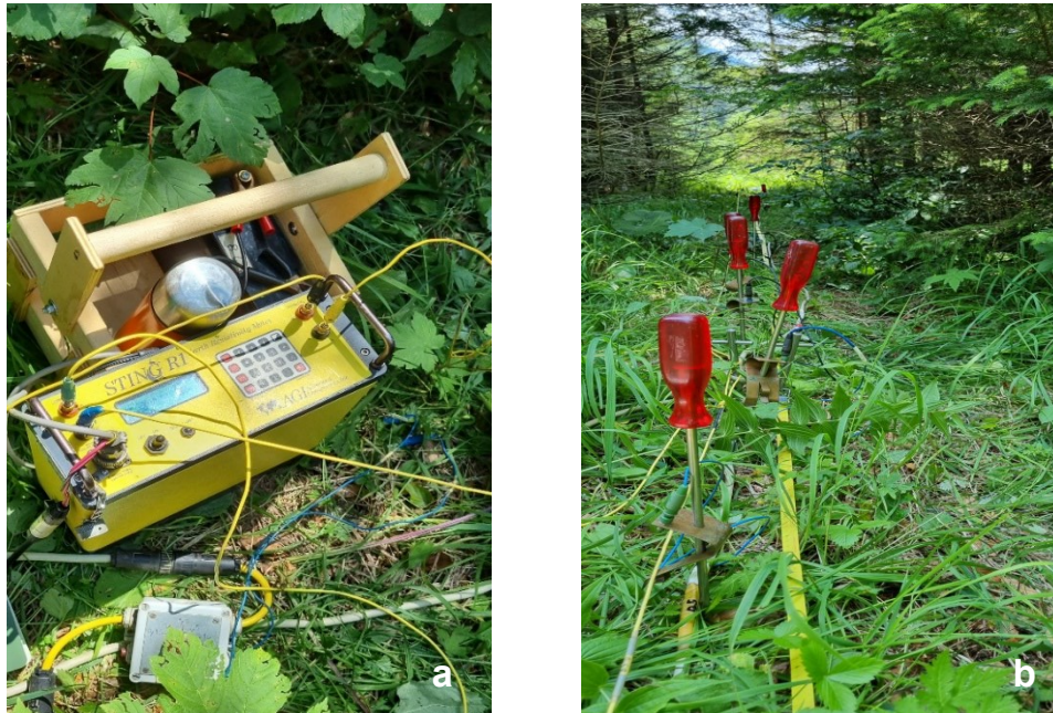
Figure 27: (a) STING R1 under real conditions. (b) Beginning of the profile hs02ves in SW direction.
