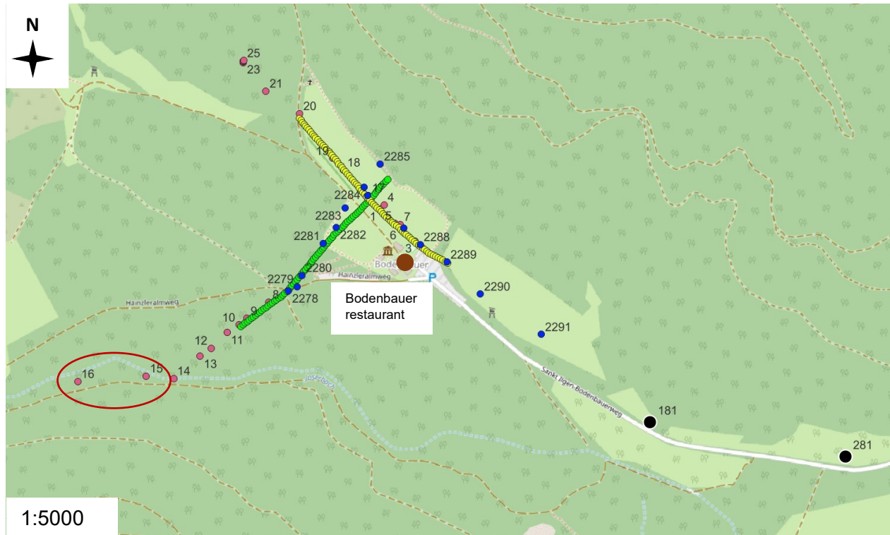
Figure 29: Position of the ERT profiles (hs01 in yellow and hs02 in green) and the VES profiles (hs01ves in red 17-25, blue 2286-2291 and hs02ves in red 8-16, blue 2278-2285). The remote electrodes for the Pole-Dipole measurements are in black. The Bodenbauer restaurant is marked with a brown dot. GPS points 15 and 16 (circled in red) depict the kink of the profile hs01ves.
