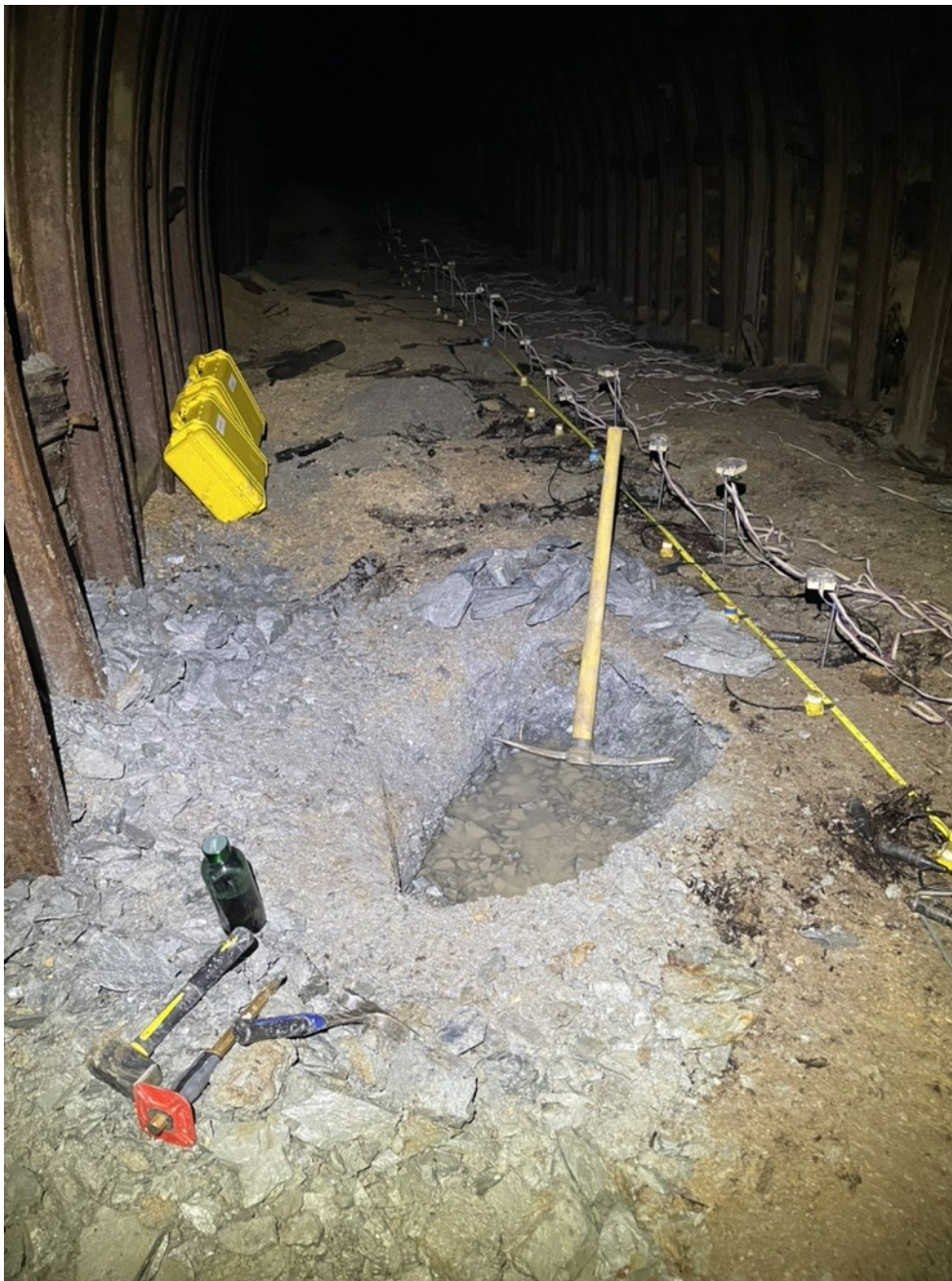
Figure 5: The hole in the foreground is sample location 5 (p5) where the solid samples were collected. The yellow measuring tape can be seen on the right-hand side of the image. The yellow devices set up along the profile are geophones. The metal spikes together with a measuring box on top are set up for the 2D ERT measurement.
