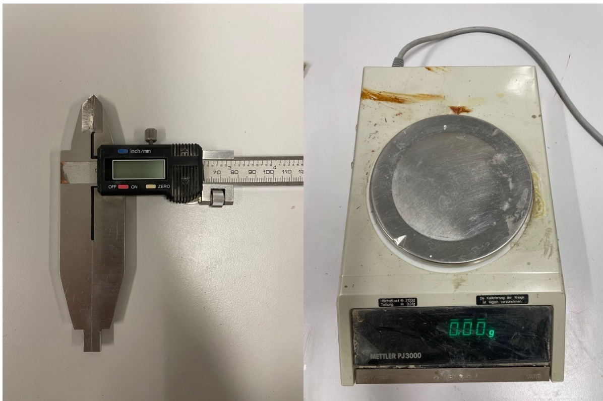
Figure 17: Left: Digital caliper slide to measure the drill core's dimensions. Right: Mettler PJ3000 scale for weighing the samples.
