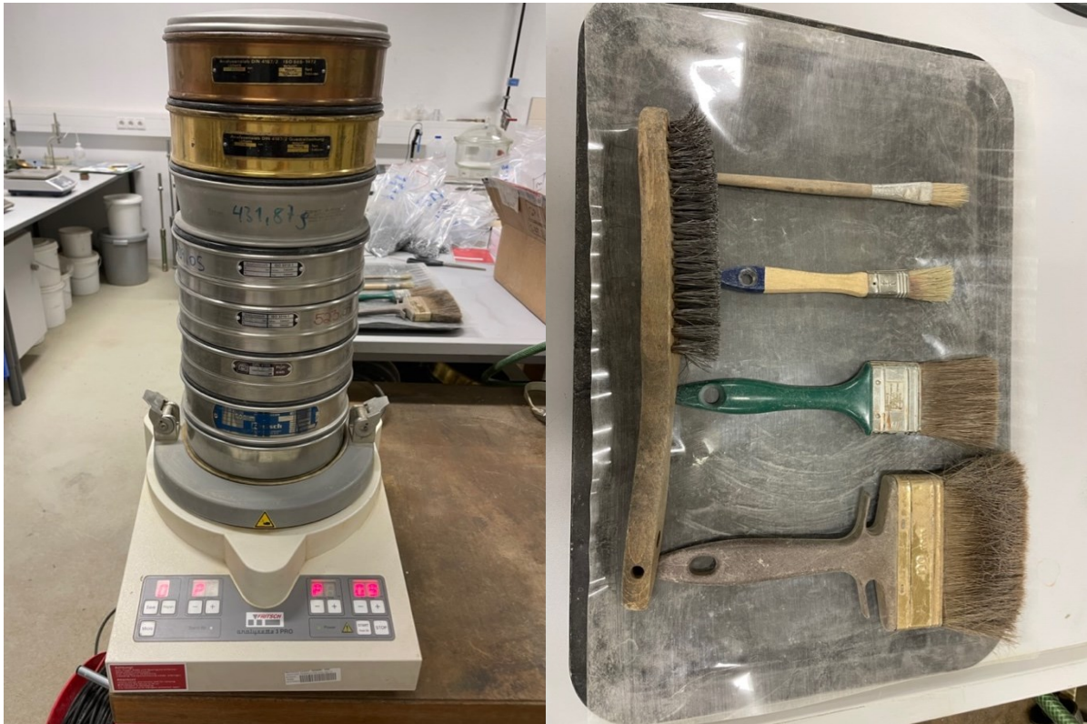
Figure 20: The equipment used to sieve the samples. On the left, the sieve tower on the electric vibrating table with the sieve sequence from bottom to top: < 500 \mu\text{m} , 500 \mu\text{m} , 1 mm, 2 mm, 4 mm, 8 mm, 16 mm, 31.5 mm. The brushes for cleaning the sieves between the individual samples can be seen on the right-hand side.
