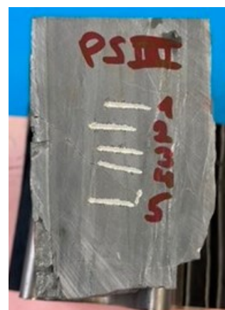
Figure 62: Picture of the sample PSIII after the CAI test. The scored areas are 10 mm long. The individual lines are numbered.
