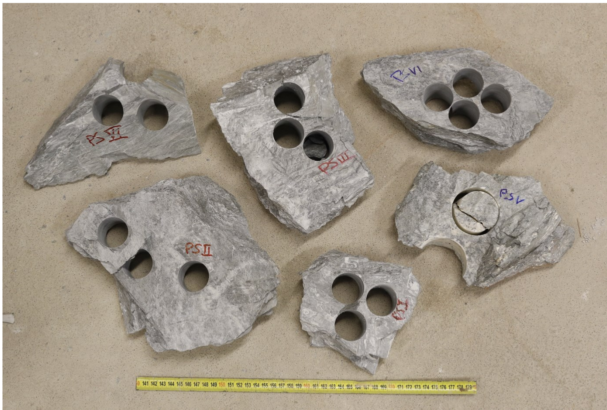
Figure 13: The six solid samples that were stable enough to drill cores from.
