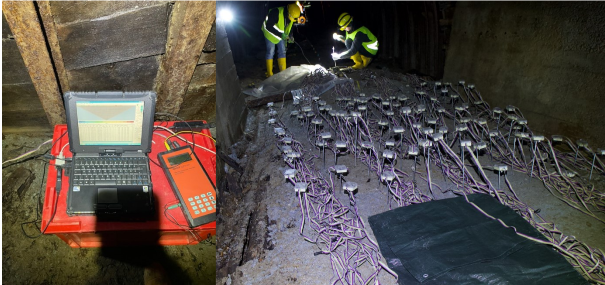
Figure 11: Left: Setup for collecting ERT data: Laptop for receiving, analyzing and storing the data. Orange "4point" device for transmitting the electrical signals and measuring them. Right: 3D - ERT array. Steel sticks, hammered into the ground with a measuring box on top, are set up in a grid.
