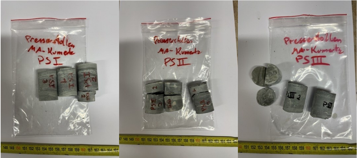
Figure 15: The drill cores obtained from samples PS I, PS II and PS III.
