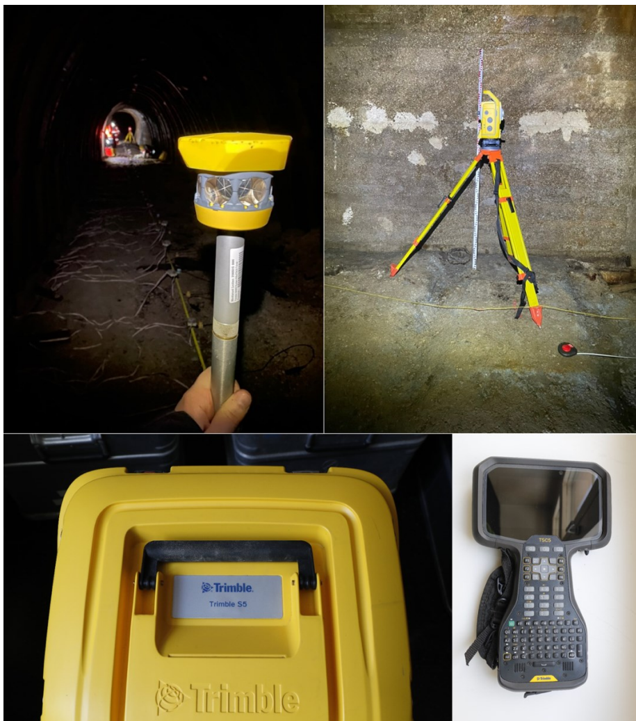
Figure 6: The equipment used during the survey: Bottom left: the "Trimble S5" surveying device in its case. Top left: the prism used for the survey, mounted on a pole at a height of 1.8 meters. Top right: the "Trimble S5" station set up with the surveying device on a tripod. Bottom right: the portable device for sending commands to the station and storing the data.
