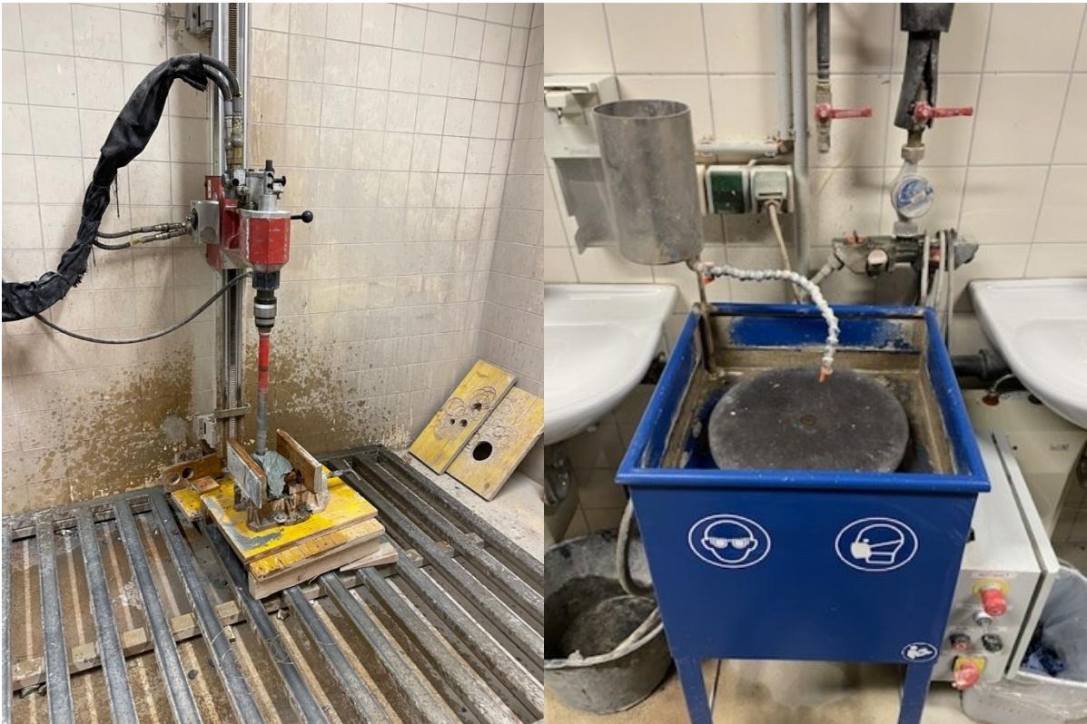
Figure 14: Left: HILTI DD-759HY drilling rig together with a drill bit with an inner diameter of 29 mm. The sample is held in place with a screw clamp and wedged with wood. Right: Spinning, abrasive plate used to polish the samples.
