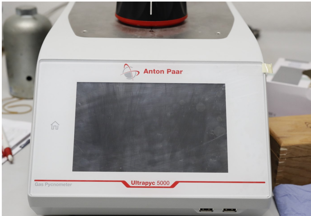
Figure 21: The Ultrapyc 5000 helium pycnometer from Anton Paar used for the measurement.
