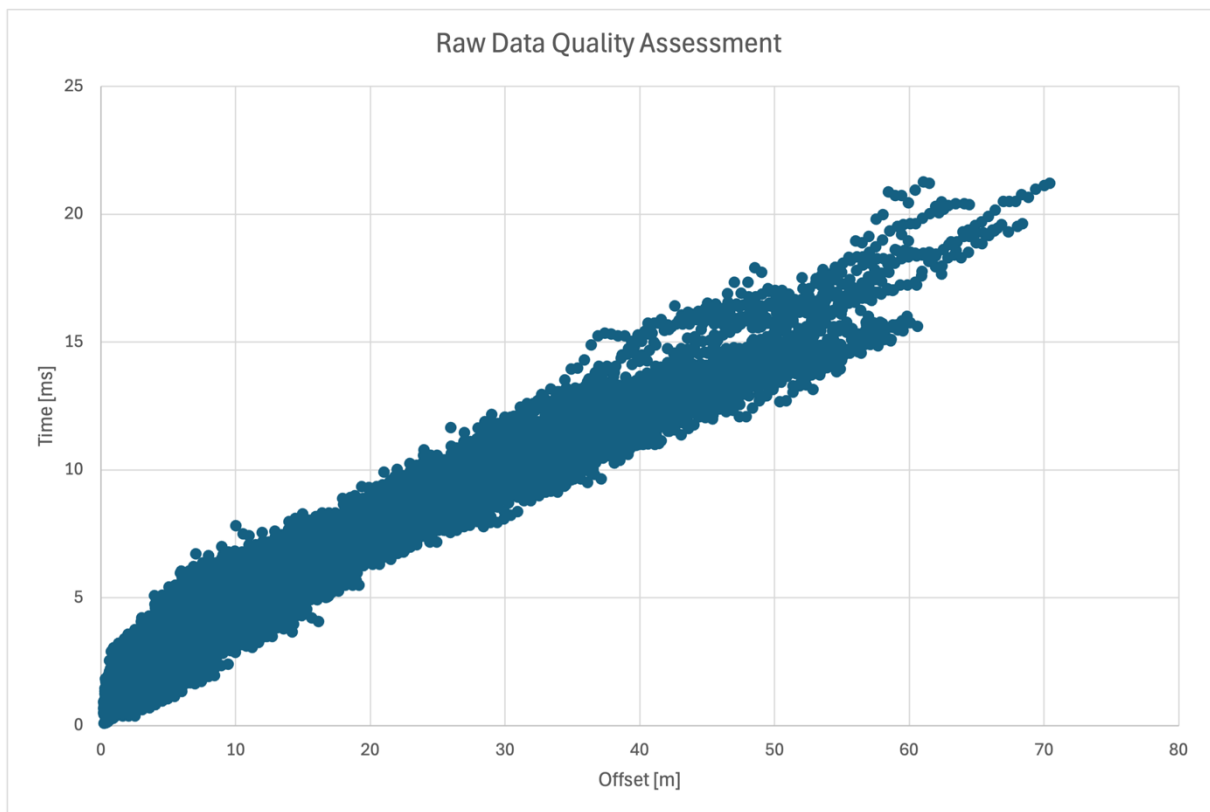
Figure 42: All seismic data points with the offset on the x-axis and the time on the y-axis to evaluate the data quality.
