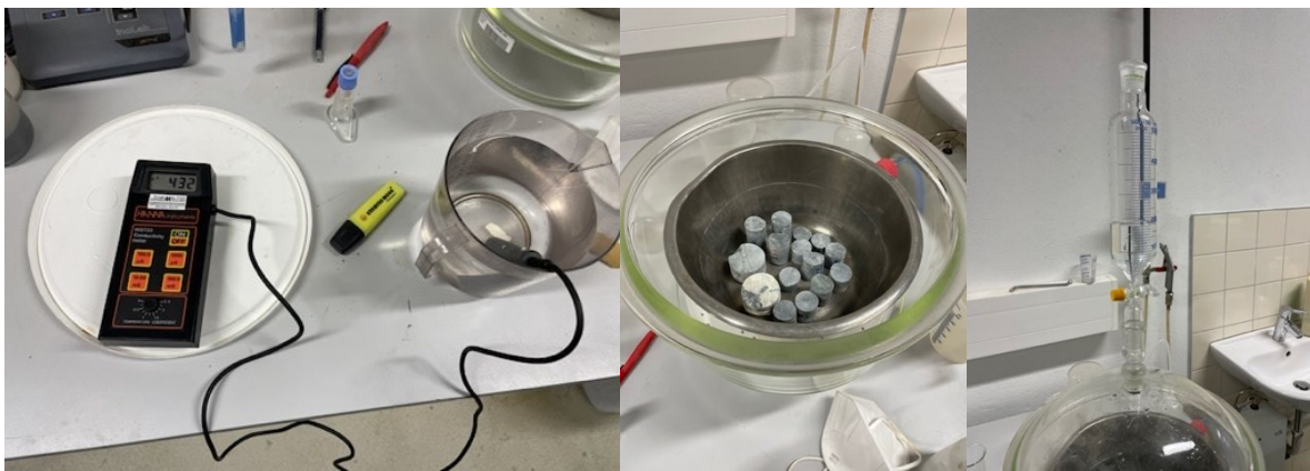
Figure 18: The devices used to saturate the samples in water: On the left, a conductivity meter from HANNA. In the center, a steel dish with the samples in a desiccator. On the right, the addition of water to the desiccator being under vacuum.
