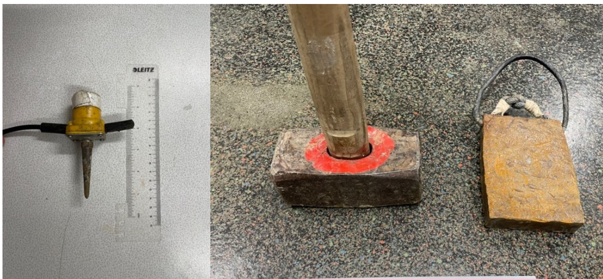
Figure 7: Left: Geophone. Right: Hammer and metal plate used for the seismic data collection.
