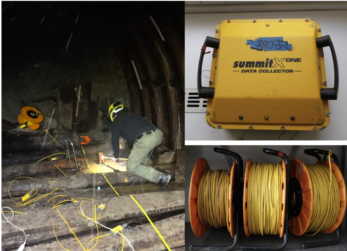
Figure 8: Left: The seismic experiment being carried out. Top right: The data collector. Bottom left: The cable drums with the data cable used.
