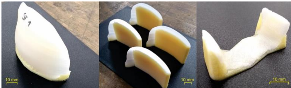
Figure 19 Benchmark “implants” printed with the optimized printing parameters (“PMMA final values” in Table 10).
