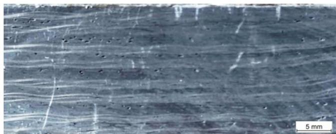
**Fig.8.2** Optical micrograph of the cross-section of the frontally cured CFRC plate obtained at a magnification of  $\times 0.65$  on a Zeiss optical microscope.
