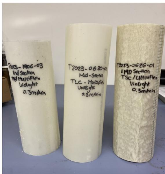
**Fig. 5.3** Left to right: Trelleborg Multiflex liners extracted from end and mid sections of a PVC host pipe cured with TRC\* and TLC\* resins. The right specimen is Ultraflex liner cured with TSC\* resin.
