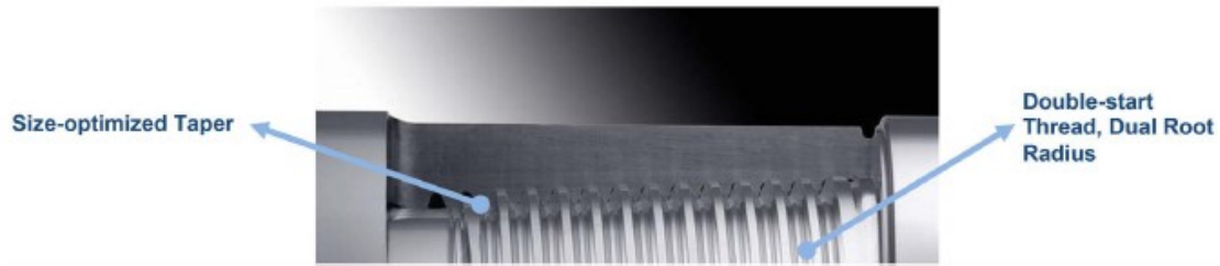
Figure 9: Third generation double-shouldered connection (Craig and Adsit, 2014).
