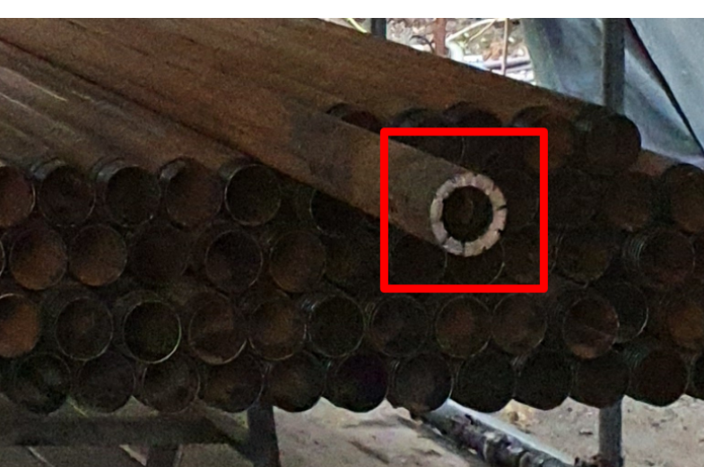
Figure 3: The drill pipes with the diamond impregnated drill bit emphasized by a red square
