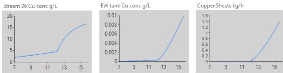
Figure 3.11: Provided graphics depicting the copper concentration in a stream and the EW tank and the produced copper sheets in ITHACA over time in hours
