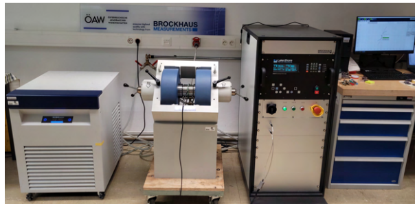
Figure 2.3.: Hystograph Brockhaus HG200 used at the Erich Schmid Institute in Leoben.
