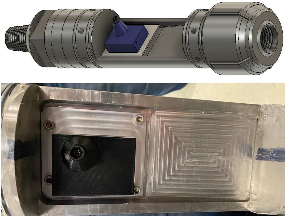
Figure 2: Prototype instrument designed to be inserted in the drill string, to enable testing under real operating conditions. Top: 3D rendering of the design. The three accelerometers and three gyroscopic sensors are contained within the blue module, together with a processing unit and Li-Ion batteries. The sensor module is autonomous. Bottom: physical prototype of the drill head used during testing.
