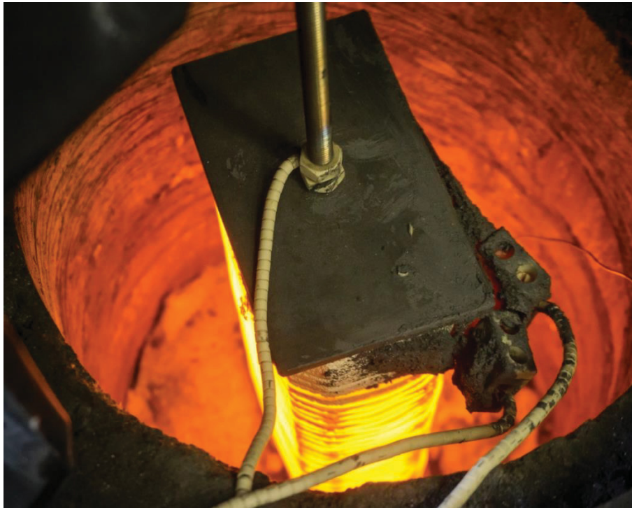
Figure 80: Preheating system for the EAF
