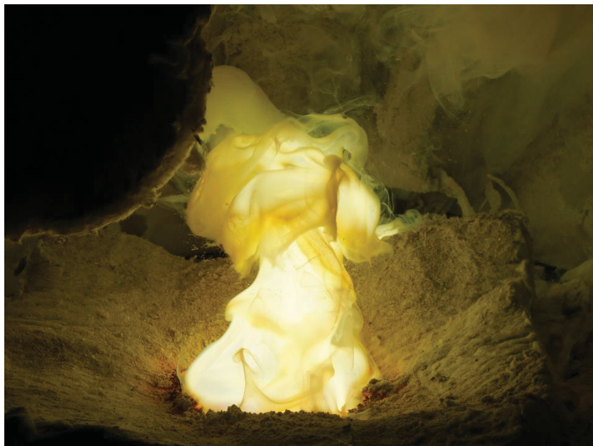
Figure 26: Re-oxidation of gaseous zinc to zinc oxide
