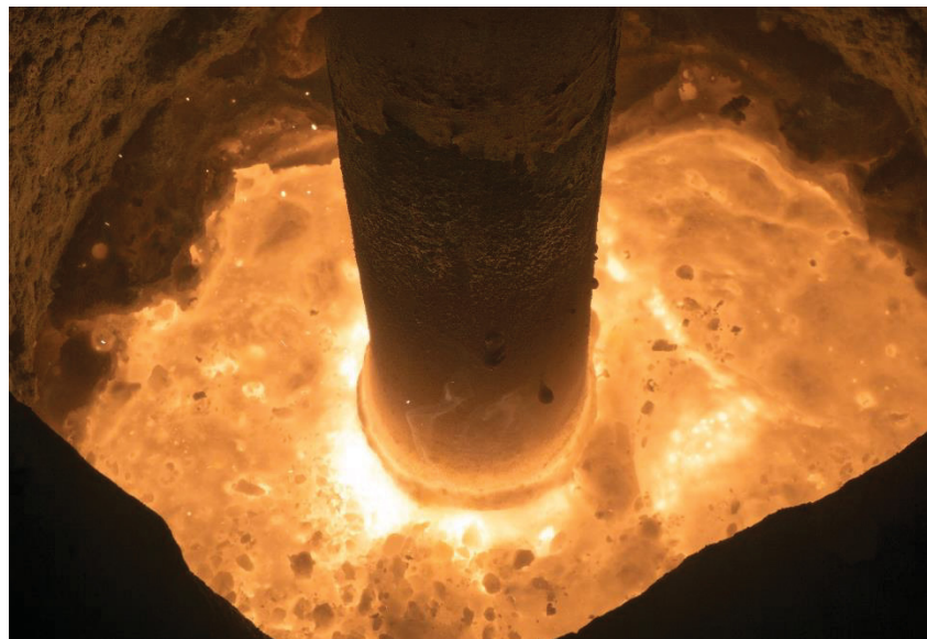
Figure 83: Inside the EAF showing a small solid layer at the top of the melt
