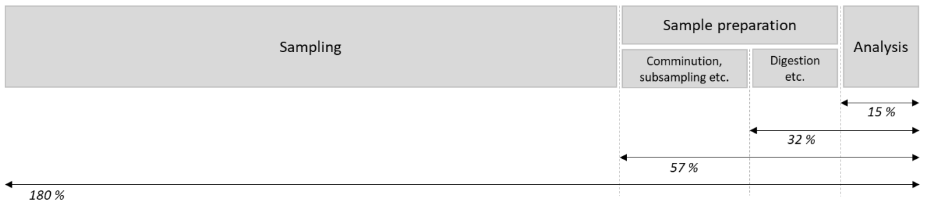
Fig. 1 Uncertainties related to the single steps of the analytical procedure at the example of lead in mixed solid waste. Adapted from Pomberger et al. (2015)
