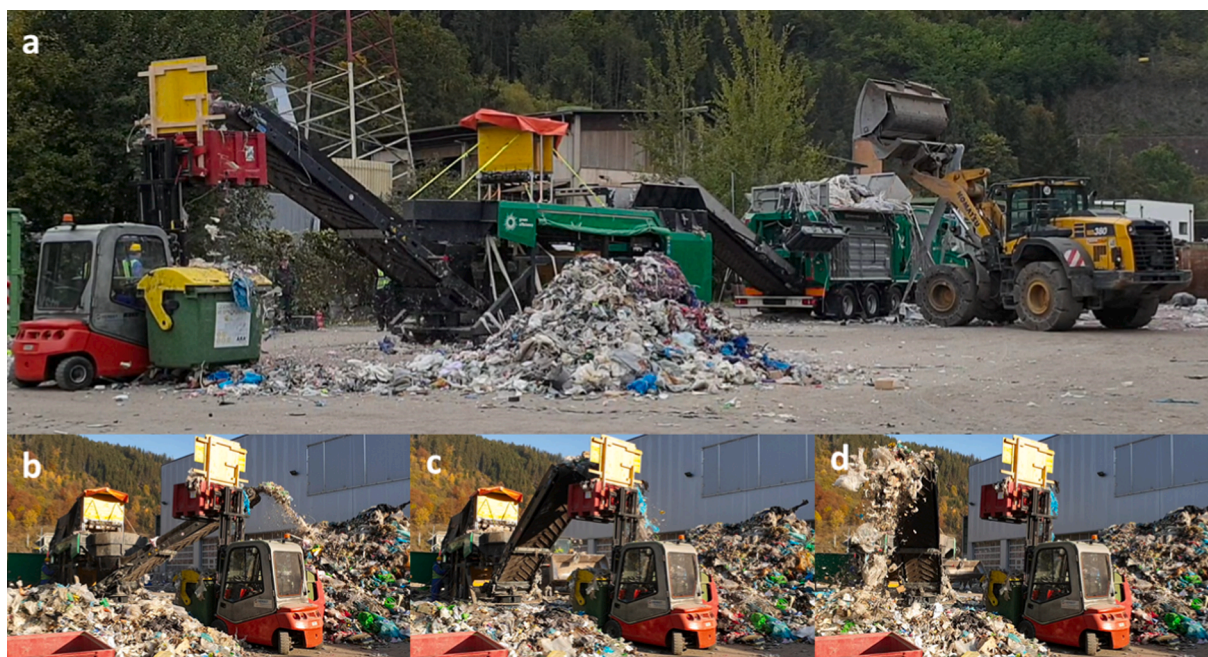
Fig. 1. a: Experimental setup of the sampling process. The conveyor belt was moved from one side to the other, i.e., from the position depicted in b via c to position d, and back to the position depicted in b, thereby sampling the waste stream twice.
