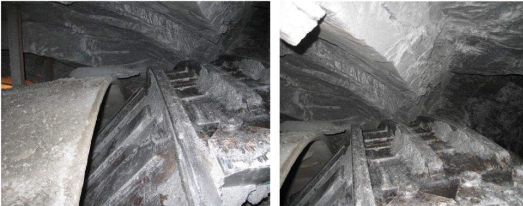
Figure 2.5: Jamming and damage of the cutterhead due to excessive fracturing of rock in a rockburst event [16]
