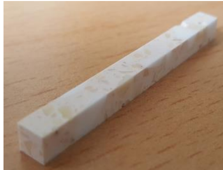
Fig. 12: Specimen used for dilatometer test.
