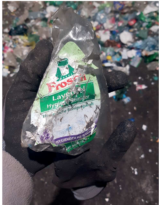
FIGURE 5: Impact of delabeller on the fully affixed paper label.
