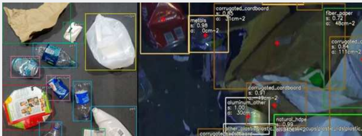
Figure 10: Classification of the material flow of a sorting robot [41,51].
