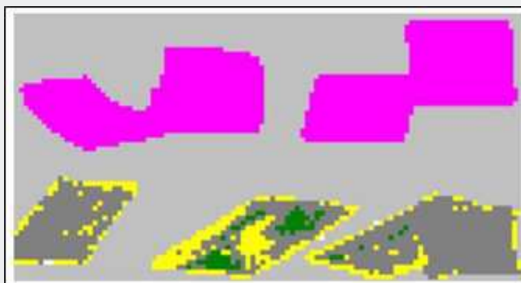
Figure 2: Polypropylene (PP) (pink) and High-Density-Polyethylene (HDPE) (grey), Non-Classified (yellow) and Polyethylene-Terephthalate (PET) (green) - Particles coloured according to their material [14].
