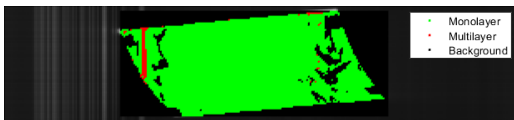
Figure 23. Classification of a PE monolayer film with the SNN.
