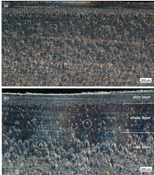
Figure 4. Polarized light microscope pictures of POM. (a) Edge of the unetched POM sample (b) edge of the etched POM sample with marked spherulites and zones.
